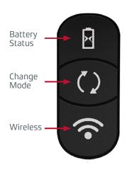
Battery Status Button: Check battery charge levels
